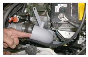
26. Slide the K&N® cold air tube into the engine compartment as shown.
