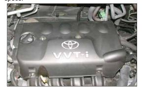
35. Install the engine cover back onto the vehicle.
