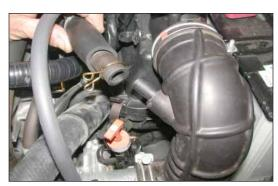
7. Disconnect the crank case vent hose from the stock intake tube as shown.
