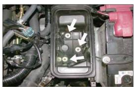
13. Remove the three screws that secure the lower air cleaner assembly as shown.
