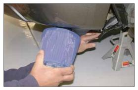
32. From underneath the vehicle pull the inner fender valance down, then, slide the air filter onto the cold air tube and secure with the provided hose clamp.
