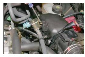
6. Use a flat blade screwdriver to unclip the vacuum switching valve from the side of the air cleaner assembly as shown.
