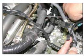
17. Unclip the two plastic wire harness clips to gain more slack for the mass air sensor electrical connection as shown.
