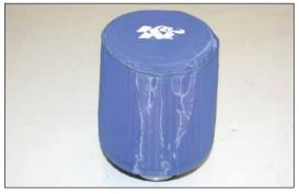
31. Install the Drycharger® onto the  $K\&N^{\otimes}$  air filter as shown.
