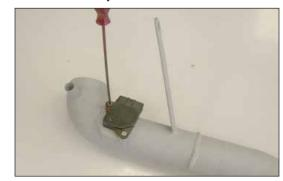
25. Install the stock mass air sensor into the K&N® cold air tube and secure with the provided hardware as shown.
