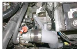
27. Slide the end of the tube into the silicone hose on the throttle body, then secure the bracket to the air cleaner mounting hole using the provided hardware as shown but do not tighten at this time.
