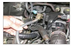
8. Unclip the vacuum hose from the crank case vent hose as shown.
