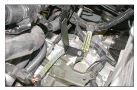
21. Install the provided "L" bracket onto the stock air cleaner mounting hole using the provided hardware as shown.
