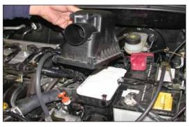
11. Release the clamps on the upper air cleaner assembly, then remove the upper air cleaner assembly as shown.
