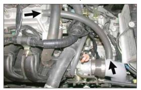
30. Install the provided silicone hose onto the vent on the K&N® intake tube, then, connect the other end to the vent on the cam cover along with the provided hose clamp.
