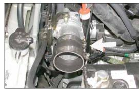
23. Install the silicone step hose and hose clamps onto the throttle body and tighten as shown.
