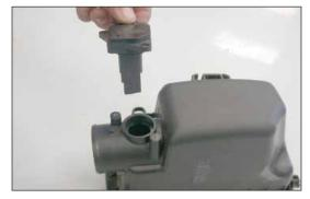
24. Remove the mass air sensor from the upper air cleaner assembly as shown.
