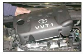
2. Remove the 4 bolt securing the engine cover, then remove as shown.
