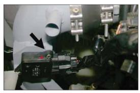
28. Reconnect the mass air sensor electrical connection using the provided hardware as shown.
