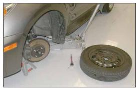
18. Raise the vehicle up and support it with jack stands, then, remove the front driver side tire as shown.
