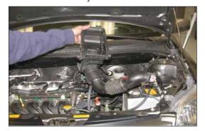
14. Pull upwards to remove the lower air cleaner assembly as shown.
