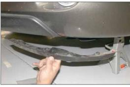
19. Remove the plastic air damn that is secured by three bolts, then remmove as shown.
