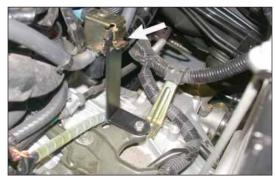
22. Slide the vacuum switching valve onto the "L" bracket as shown.
