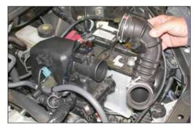
10. Loosen the hose clamps at the throttle body and at the air cleaner assembly, then, remove the stock intake tube as shown.
