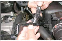
5. Remove the tape that binds the mass air sensor wire harness to the vacuum switching valve wire harness as shown.
