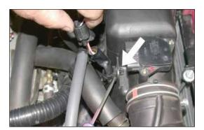
4. Using a flat blade screwdriver unclip the wire harness as shown.
