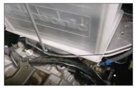
16. Using a cutting tool, trim the plastic battery tray to mirror the inner fender as shown.
