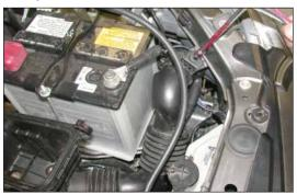
12. Remove the bolt that secures the air inlet duct as shown.
