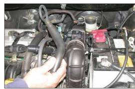
9. Disconnect the crank case vent hose from the cam cover, then, remove the crank case vent hose as shown.
