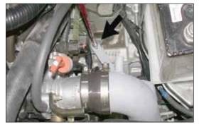
29. Adjust the tube for best fit then tighten the bracket and the hose clamp as shown.
