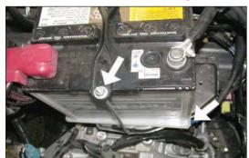
15. Loosen the battery hold down bracket and slide the battery as far towards the fender as possible.
