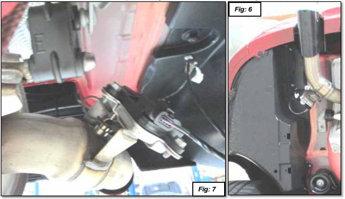
7. Remove the 3 screws and 1 nut holding the left inner body side cover and let it hang down to give you access to a spot to zip tie the valve out of the way as shown in figure. Position the actuator with the wire connector
