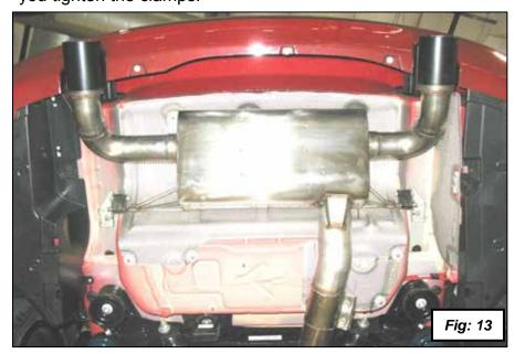
If the muffler has holes for a locking clip on the hanger the end of the clip should face forward. If you have the hangers with the 90° bend shown on the previous page you can ignore this.
