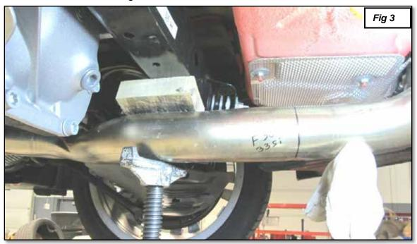
4. This step applies to 435i and xDrive only; skip to step #6 if you are working on a 335i. For a 435i find the BMW factory punch mark on the exhaust. Measure ¾ of an inch from the punch mark toward the back of the car and cut at that point.
