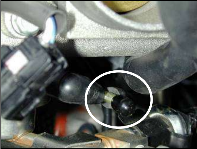
d. Install supplied vacuum cap onto the open port on the vacuum fitting.
