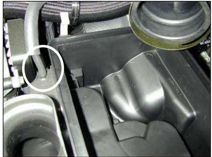
f. Pull vacuum hose off of the nipple on the air box.
