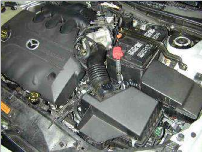
a. Stock air box system installed.
