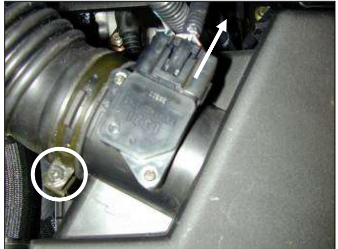
b. Unplug MAF sensor and loosen hose clamp at air box inlet.
