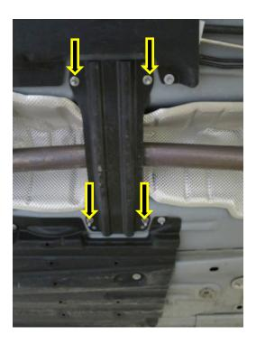
4. With the brace removed, use a 15mm box wrench to break loose the nuts that secure the downpipe to the exhaust system.
