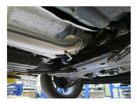
2. Working your way back, loosely install the up and over pipe to the forward pipe using a supplied gasket and supplied nuts and bolts.
