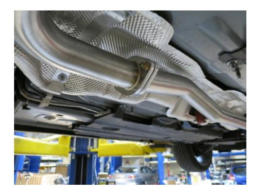
3. Repeat the same step, using the supplied gasket and bolts, to install the rear muffler section onto the car using the factory exhaust hanger bushings.
