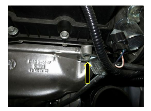
13. With a 10mm socket, using an extension and universal joint, reach down the back of the motor and locate the upper-most downpipe bolt that holds the downpipe to the turbo. Compare the mounting pattern to your COBB downpipe to get an idea of where you'll need to reach. You'll need to push the heat shield out of the way to gain access. Depending on your tools, you may also have access to the second bolt towards the passenger side of the flange.
