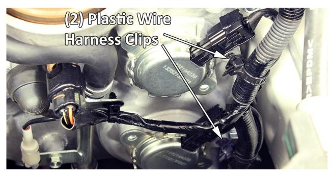
b. For 2022+ models, locate plastic wire harness holder as shown in picture below. This is held onto the engine using some built-in one-way plastic fasteners (Christmas tree fasteners). Using proper tools, slowly pry away from the engine taking note of the location of all the plastic one-way fasters. Once harness is freed from the engine, install PERRIN Cam Solenoid Guards under it. After they are installed, simply push plastic wire harness back into the holes on the engine.
