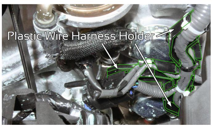
Reinstall plastic clips back into the holes they were installed in. If extra plastic wasn't trimmed off enough, they may be slightly hard to install, and additional trimming may be needed.
