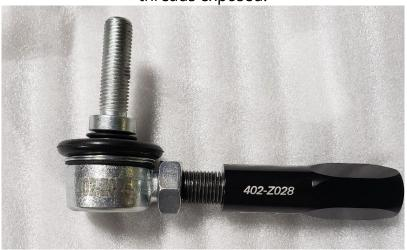
\*You are now ready to start the installation process. Use the length of the stock component as a starting point for the length of the 034 adjustable end links; expand or compress as best fits your needs
