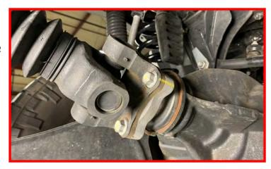
Carefully remove the larger clamp on the front driveline dust boot. Slide the boot back to gain access to the retaining clip.
