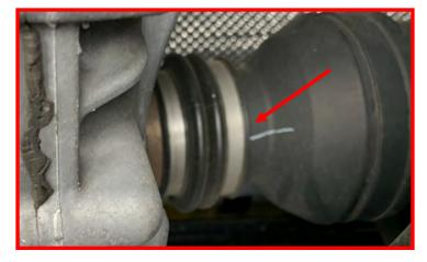
Using the appropriate pliers, open the retaining clip and slide the front driveline off the splines.
