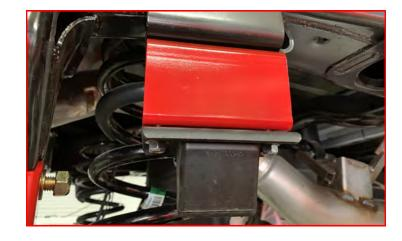
Install the replacement rear shocks using the factory hardware on the bottom and the provided hardware on the top of the shock. Do not tighten at this time.
