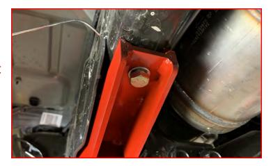
Rotate the axle until the radius arms are lined back up into the drop brackets. Install using M18 bolts, washers and nuts.
