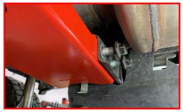
Install (3) supplied M12 bolts, (3) locking nuts and (6) flat washers through the rear holes on the transmission mounting plate, mounting plate spacer and the transmission crossmember. Do not tighten at this time.
