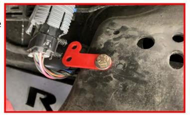
Install the harness connector onto the relocation bracket.
