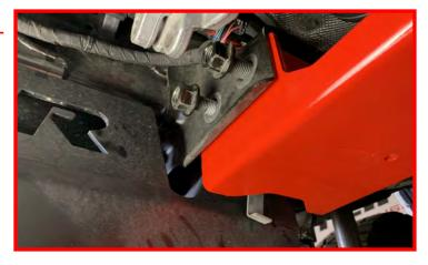
Using the factory transmission crossmember hardware install the passenger side from front to rear. This will aid in removal if service needs to be performed.
