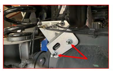
Loosen but do not remove the upper and lower control arm bolts on the axle and the frame pockets.
