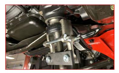
Note: Be sure to thoroughly clean splines prior to installing pitman arm.
