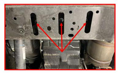
Remove the (3) transmission mounting nuts and retain the factory nuts.
