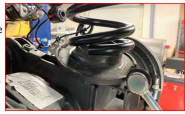
Passenger side ends up with end of the weld on the lower cup to axle/track bar mount. This is necessary to keep the springs matched to the angle of the mounting cups on the axle. Failure to do so will cause the springs to bow out in inappropriate angles.
