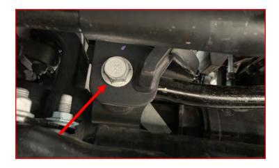
Remove track bar hardware at the frame and swing track bar out of the way.
