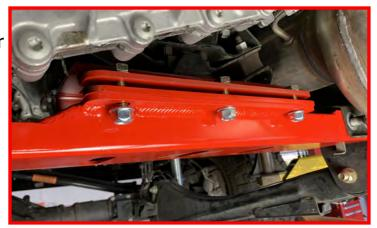
Install (3) supplied M12 bolts, (3) locking nuts and (6) flat washers through the front holes on the transmission mounting plate, mounting plate spacer and the transmission crossmember. Lower the transmission down on top of the mount.
