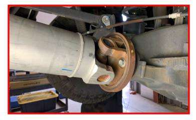
Using the factory hardware and thread locker, install the drive shaft to the pinion flange lining up the previous marks.
