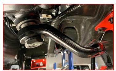
Loosen tie rod end adjuster and rotate tie rod end 180 degrees. Attach tie rod end to pitman arm using factory hardware.
