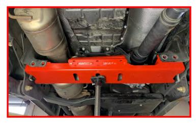
Using the factory transmission crossmember hardware, install the driver side from front to rear.
