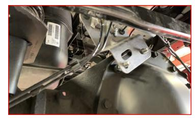
\*\*\*Note: Some models have a torque shock located on the differential. This will need to be removed for the function of this kit. \*\*\*
