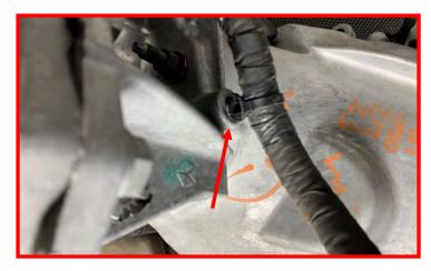
Remove the harness connection from the driver side transmission crossmember mounting.
