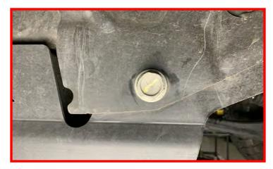
Remove the driver side transmission crossmember bolts and retain factory hardware.
