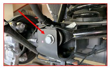
Remove the upper track bar mounting bolt.
