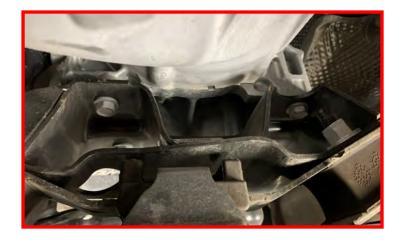
Tighten the transmission mount bolts.
