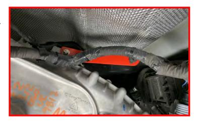
Install the transfer case shift solenoid connector.
