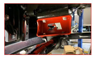
Install brake line drops to the brake line bracket using 5/16" bolts, washers and nuts. Do not tighten at this time. Attach brake line and drop bracket to the inside frame rail using the factory hardware. It will be necessary to gently pull down and bend the metal brake line on the driver side to gain the slack needed.
