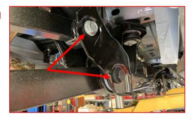
Lower the axle just enough to remove the springs.
