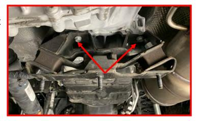
The remaining (2) bolts are located at the front of the mount. Remove the (2) bolts and remove the mount. Retain the factory hardware.
