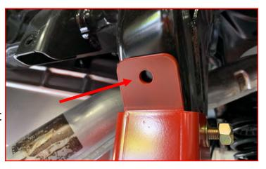
Install rear coil spring spacers using 3/8" bolts, washers, and c-lock nuts.
