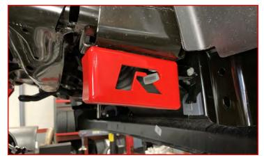
Install the sway bar to the drop brackets using 7/16" bolts, washers, and nuts.
