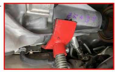
With the transfer case supported, locate the (3) transmission mounting nuts.
