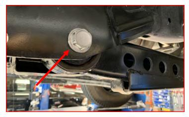
Mark the driveshaft to pinion location. Remove the front driveshaft from the axle. Let hang out of the way.
