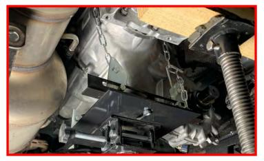
Remove the (6) transfer case mounting nuts. (2) are located on the bottom, (1) on either side on the transfer case and (2) located on the top.
