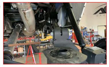
Install track bar bracket using the 14mm x 110mm bolt, washers, and c-lock nut and crush sleeve in the track bars original location.
