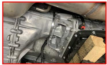
With the transfer case installed and mated back to the transmission, installed the (6) supplied 3/8" locking nuts and flat washers.
