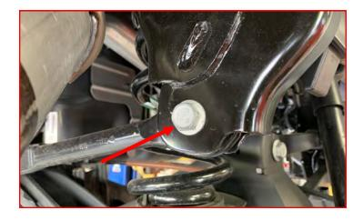
Remove parking brake bracket mounting bolts from the lower control arm on the driver side. Retain hardware.
