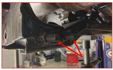
Note: Vehicles that are equipped with optional diesel engines, It will be necessary to raise the DPF (Diesel Particulate Filter) to remove passenger side transmission crossmember bolts. The following steps will instruct you on how to proceed.
