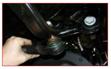
Loosen but do not remove track bar bolt at the axle.
