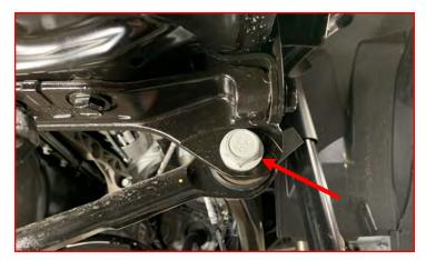
Lower the axle enough to remove the coil springs from their mounts and discard. Be sure to retain the factory spring isolators.
