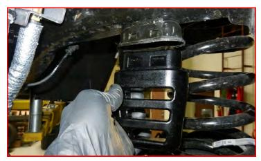
Using an appropriate cutting tool, remove the alignment tab. It is necessary to trim the tab off the coil spring isolator for install.
