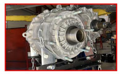
Once the transfer case is removed from vehicle, remove the factory mounting studs. There are two was to remove the studs.
