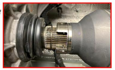
Mark the driveshaft to pinion flange location. Remove the rear driveshaft hardware from the flange. Let hang out of the way. Retain the factory hardware.
