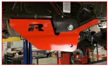
Locate the (4) wire flag nuts and the (4) holes on the outside of the frame. Bend the wires to align the tab nut with the rear mounting holes in the bracket and frame.
