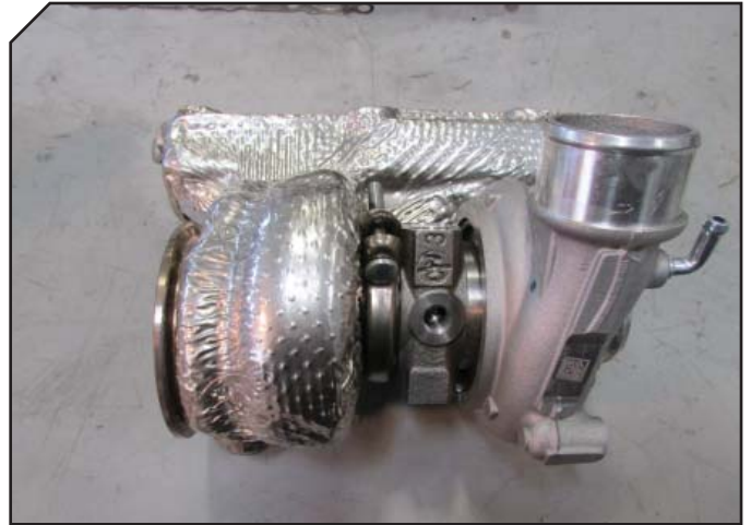
INSTALL HEAT SHIELD
