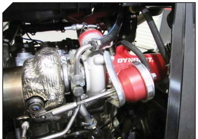
INSTALL WASTEGATE ACTUATOR
