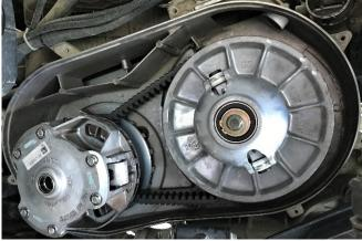
11. Once primary is torqued, with transmission in PARK, spin secondary clutch back & forth a few times to allow belt back to top of secondary.
