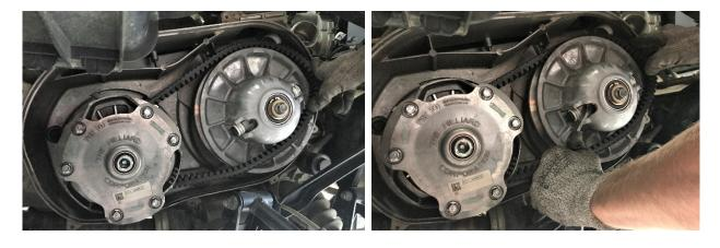
13. Install outer clutch housing. Ensure seal is good or replace.
