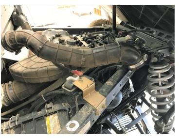
2. Remove the clutch housing cover. Recommended tool: 8mm socket with flex drive extension.
