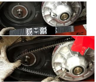
10. Slide belt into DURACLUTCH DCR Primary clutch then install on post. Use NEW primary screw, steel bushing and plastic bushing. Note: Plastic bushing goes inside of primary post and steel bushing will be on outside of post. Torque primary screw to 47 ft-lbs.
