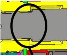
5. Install the NEW M8X1.25X75mm secondary screw, lock & domed washer provided with kit. Discard any other washers. Place Blue Loctite provided on the secondary screw threads. Tighten screw to 27 ft-lbs.
