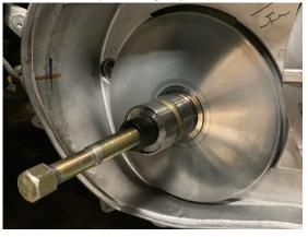
8. Clean the engine tapered shaft and Primary clutch bore with alcohol or degreaser. Do not lubricate.
