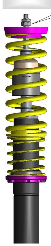
Install the factory top mount and secure it with the supplied nuts. Tightening torque for the piston rod nut is 20 Nm (15 ft-lb). The strut unit has to be installed according to manufacturers instructions settings regarding tightening torque and fixing specifications.
