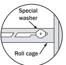
The special washer is placed on the figure of the Roll cage
