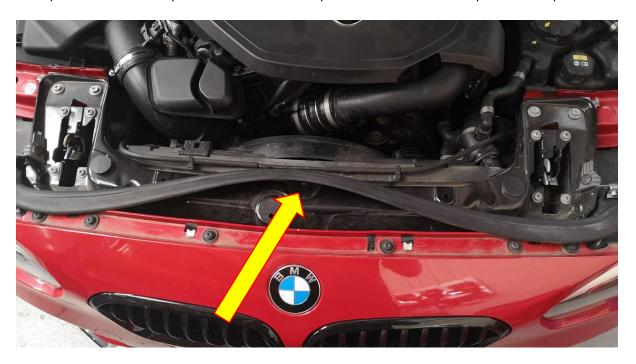
2. Using a T30, undo and remove the x6 bolts. You can then pull the bumper gently towards you to release it from x4 catches that locate it.
