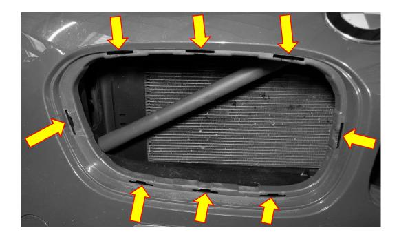
5. With the bumper now slightly loose at the top, gently pull it towards you to gain access to the top clips that hold the kidney grills in place. Depress the centre of the tab downwards, then push the clip so that it slides under the bumper (therefore releasing it).
