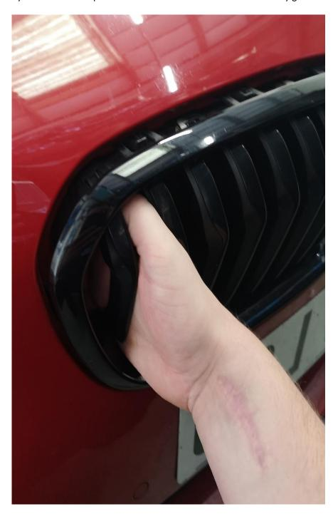
8. To release the final 3 tabs along the bottom, reach your hand through the slats and use your finger to depress the centre of the tab in the same method as previously used, again gently pull on the kidney grill surround to release it. Repeat this until all three are loose, then you can pull the whole kidney grill towards you to remove it.
