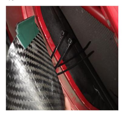
13. Remove the backing off the double-sided tape. Line up FMINLD2 inside the opening, with the cable ties going around the support bar. Hook the end of FMINLD2 around the corner of the opening and push firmly for 30 seconds to ensure good adhesion.
