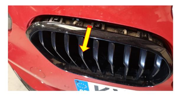
7. Slide your hand in between the final few slats on either the left or right side of the kidney grill and reach for the singular tab on the side. Depress the centre of the tab in the same way as the previous step, and then use your other hand to gently pull the kidney grill surround towards you to release. Repeat this for the other side of the same kidney grill.
