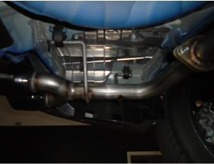
**Step 2.** Next loosely install both Tail Pipes by bolting the inlets flanges to the Y-Pipe Assembly using the OEM hardware and supplied gaskets. Insert all welded hangers into the OEM rubber insulators.
