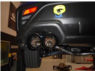
**Step 3.** Once a final position has been chosen for the new exhaust system, evenly tighten all clamps from front to rear using the torque specification on page one of these instructions. Inspect all flasteners after 25-50 miles of operation. Re-tighten if necessary.
