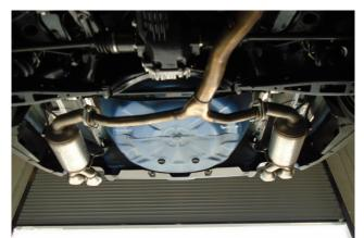
**Step 1.** Remove both muffler assemblies by unbolting them from OEM Y-Pipe assembly. Remove all welded hangers from the rubber insulators. Retain all mounting hardware as it will be needed to install your new MAGNAFLOW system.
