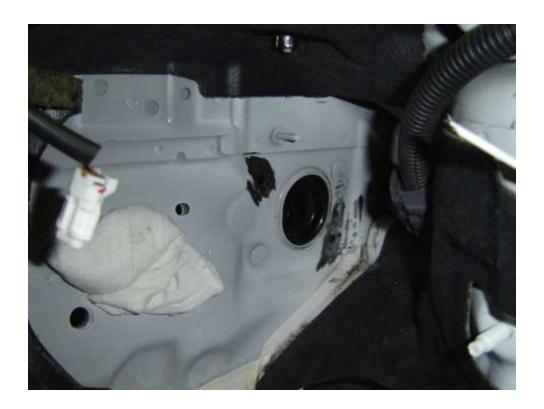
7. To prevent rust and corrosion touch up the bare metal around the holes with paint. Spray paint would be an ideal choice here, be cautious of overspray.
