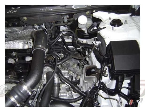
2. Now remove the brake master cylinder. Start by disconnecting the fluid level sensor connector. Then the two hard lines going to it. And finally the two 12mm nuts and pull off the master cylinder. Notice that there is an o-ring between the master cylinder and brake booster. This has to go back on later or you will end up with a large vacuum leak. Make sure to put a lot of shop towels below the master cylinder to soak up the brake fluid and be sure to keep it off of all painted surfaces.
