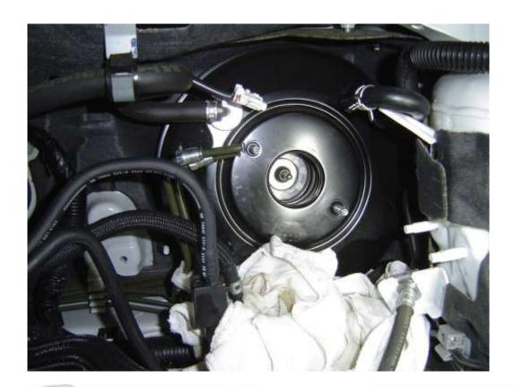
3. At this point you can remove the brake booster. Begin under the dash and remove the 4 nuts holding it to the firewall. And then remove the clip and pin holding it to the brake pedal. While under here pull the clutch master cylinder shaft off of the clutch pedal also.
