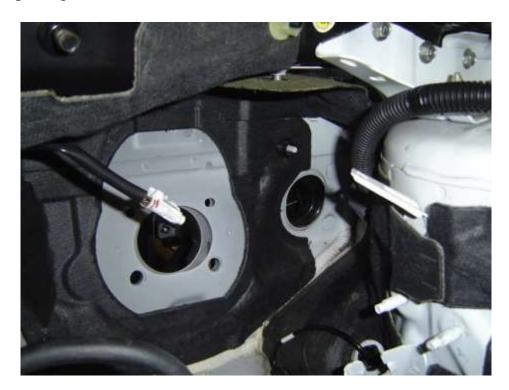
6. Now it's time to pull out some sort of grinding tool that can fit in tight spaces. You will have to grind off the backs of the top-left and bottom-right studs around the clutch master cylinder. These are marked with an X below. Be careful not to grind into the firewall sheet metal. As you get deeper you will begin seeing and outline of the stud. At some point you will be able to push the stud out leaving a clean hole behind.
