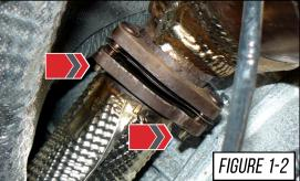
The remainder of the removal process takes place under the car. Removing the belly pan is accomplished by removing the fasteners as shown by the arrows in **Figure 2**.
