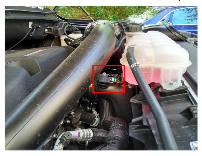
Attach the brown connection to the MAP sensor shown below. Finally, route the cables and place the control box next to the battery.
