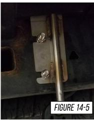
Install the rear axle tubes, Drivers side (part C19) and passenger side (part C20). Use the supplied 3.0" Accu-Seal Clamps (a) and rubber exhaust isolators (b) shown in Figure 15.
