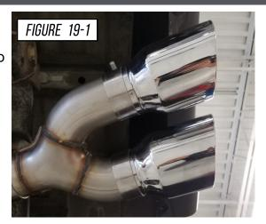
For dual side tip outlets, use the supplied 3-inch Accu-Seal Clamps (TAS300) to install the 5" straight cut tips to the same specifications outlined in **Step 9**.
