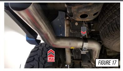
Install the exhaust hanger split collars and included Allen wrench to help keep the exhaust system aligned and secure. Install these clamps in the orientation shown in **Figure 18**.
