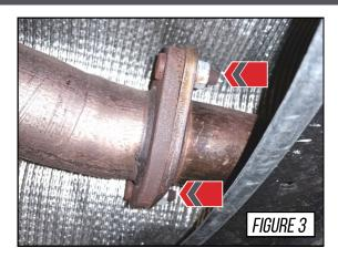
Install the non-resonated front section (part **ZR**), reusing the factory gasket and supplied M8 hardware.
