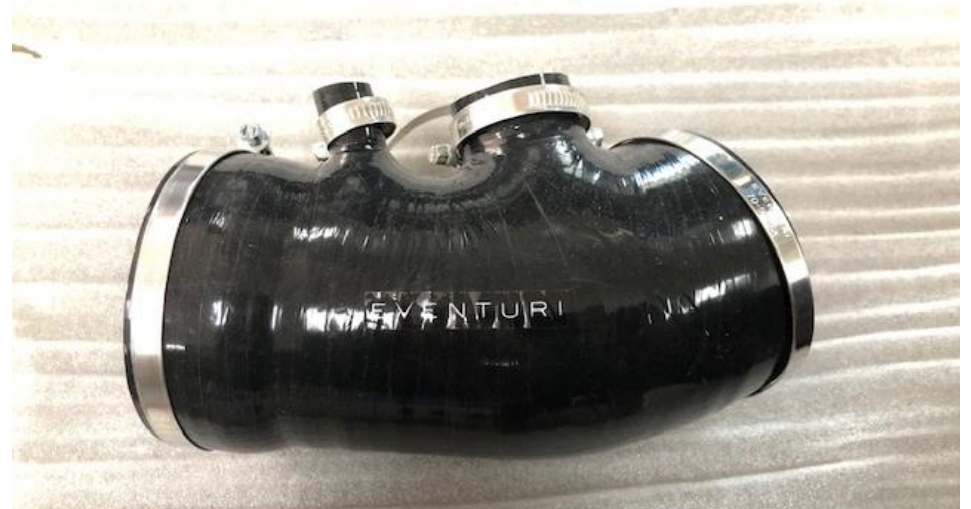
34. Take the new Silicon hose and use the 2 small hose clamps and the breather boss from your previous silicon hose removed from the intake (removed in step 2).
