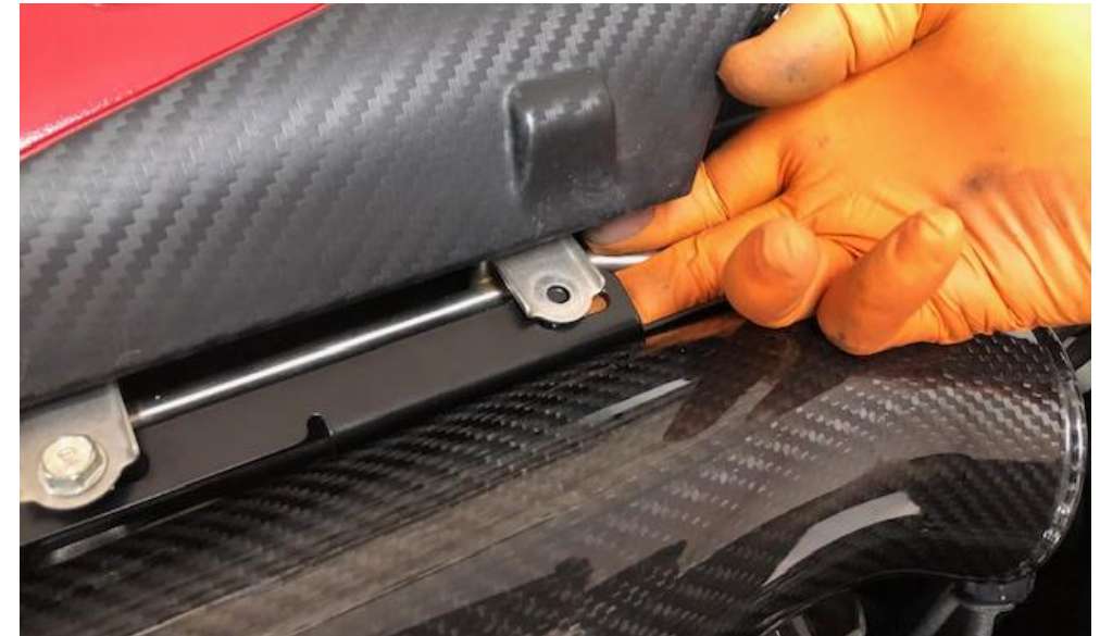
30. Use the 2 x M6 x 16mm bolts supplied with the 2 x M6 lock nuts to secure the metal line to the bracket.
