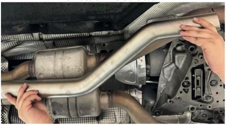
**Step 3:** Mark where you're cutting with a sharpie. We recommend 45mm or 1.75" from the hanger bracket. Use a pipe cutter to make a clean cut. If handy, use a file or debur tool to clean the cut further.
