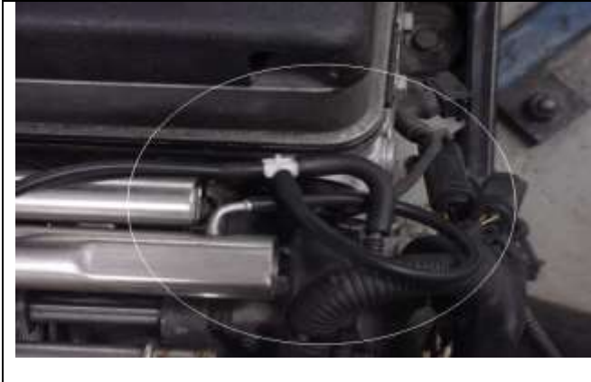
34. LOOP VACUUM LINE AROUND TO PRVENT KINKING.
