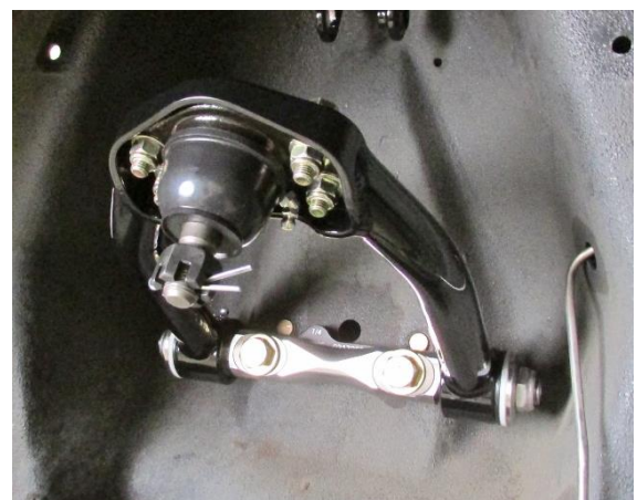
Figure 13 - Install Upper Control Arms
