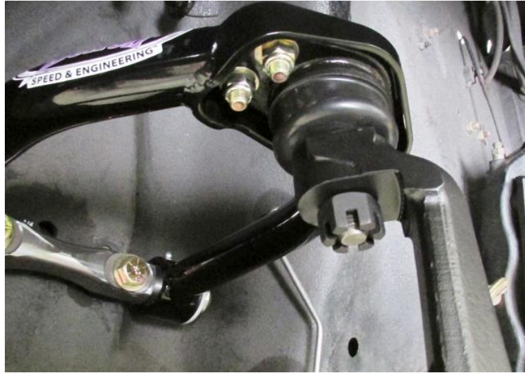
Figure 22 - Install Upper Ball Joint
