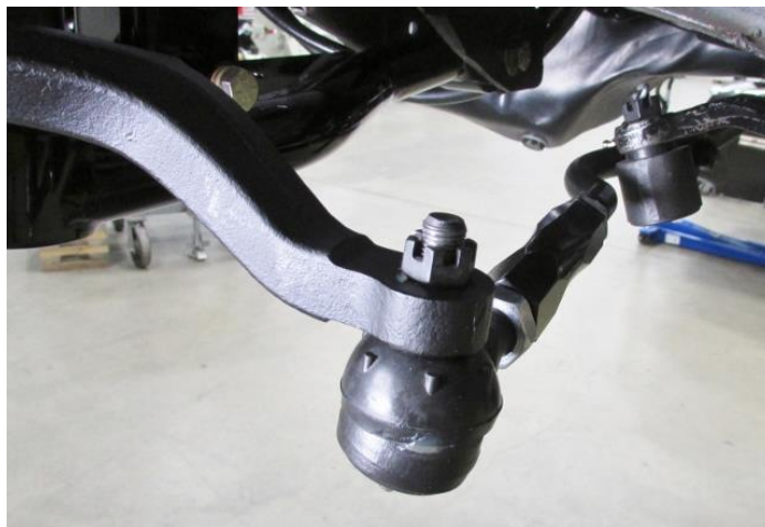
Figure 26 - Install Outer Tie Rod
