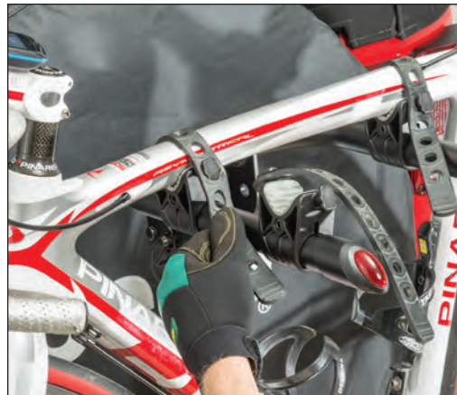
Pull the rubber retaining straps over the frame of the bike and secure it on the rectangular hook.
