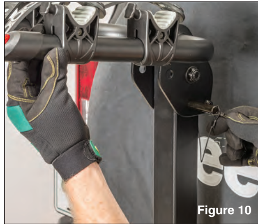
into place. Reinstall the pin and retaining clip into the lower hole.
