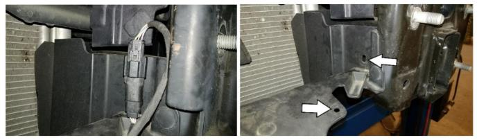
8. Unbolt the bumper by removing the (2) 8mm bolts, *one on each side*, front splash guard bolts and (6) 21mm bumper nuts, *three on each side*.
