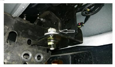
2. (*Diesel*) Remove the bracket the attaches the air dam to the frame. Also, remove the rectangle tubing from the frame.
