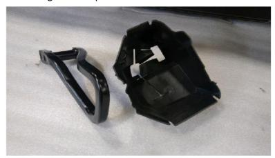
5. Also remove the tow hook trim panel. It is mounted by two 7mm screws and one clip.
