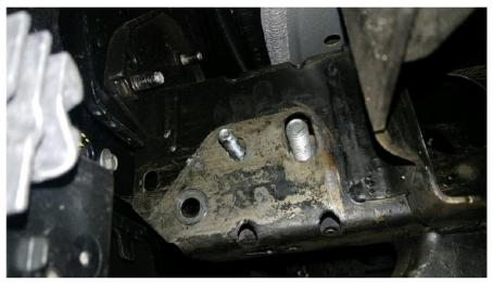
8. From the back side, slide the mounting bracket through tow hook opening. Use 3/8" and ½" washers, lock washers and nuts to install.
