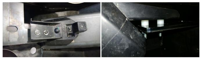
10. Install the bumper buy using the  $\frac{1}{2}$ " hardware provided. You will use the inner holes.
