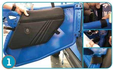
Place the Door bags on the door as shown, and secure the top two(2) Velcro straps and the strap on the front tube, as shown.
