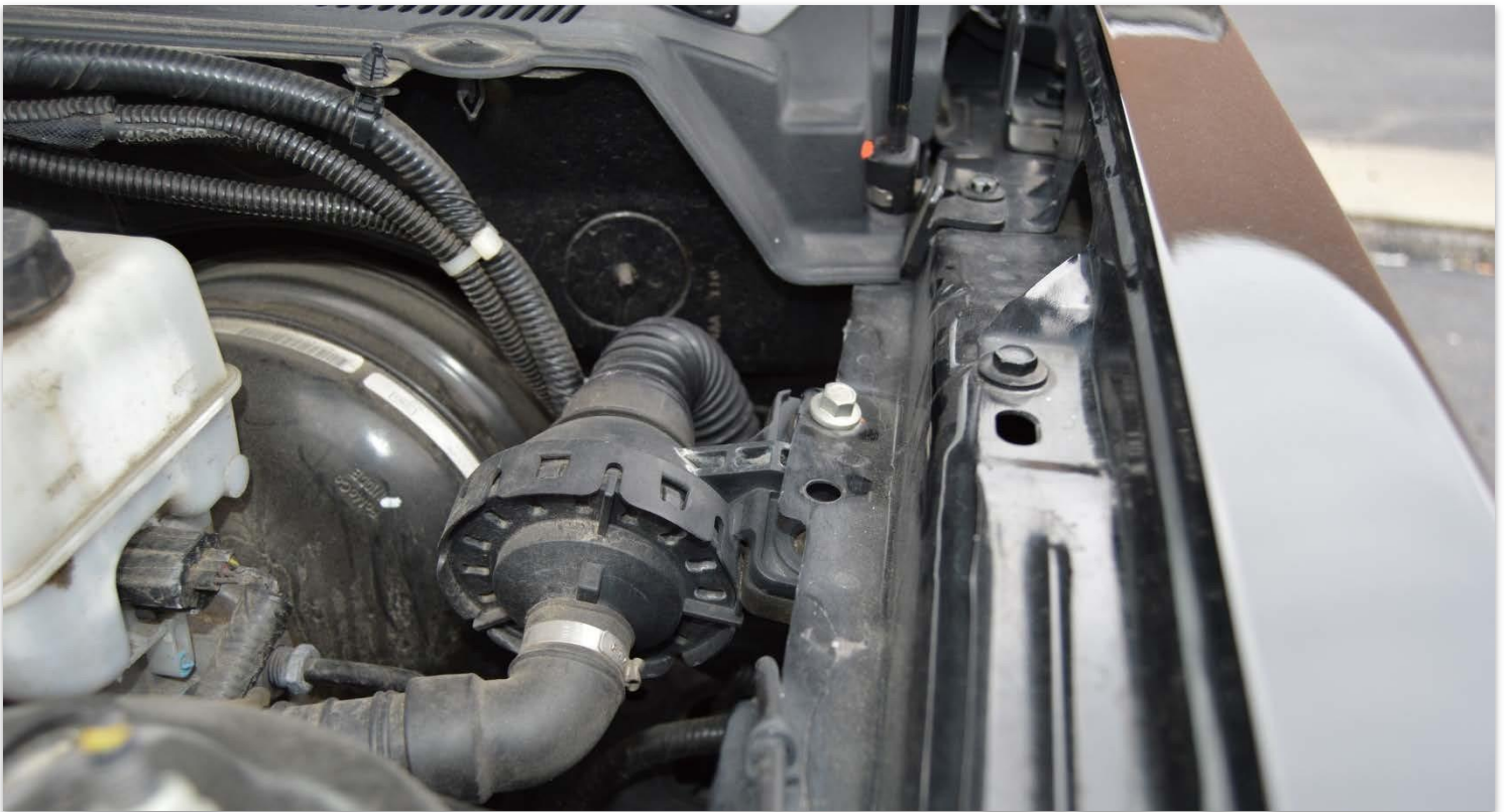
View of sound canister after relocation:
