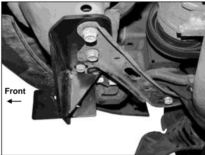
(Fig 3) Passenger/right Mounting Bracket installed
