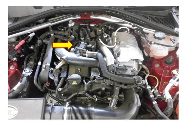
3. Using an 8mm socket and ratchet with extension remove the X3 OE fasteners attaching the OE dump valve to the boost pipe.
