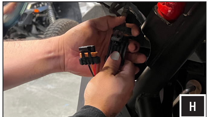
H. Unplug the factory tail light connector and plug it to the "PASS. INPUT" connector of the X3 Rear Turn Signal Harness (B-H3205).
