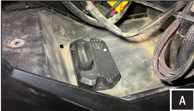
A. Mount the module to the front section of the center console behind the start/stop switch.
