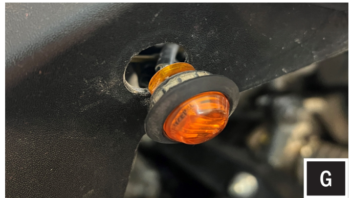
G. Insert the LED turn signal lamp into the hole and push in to lock in place. Repeat steps F and G for the other side.
