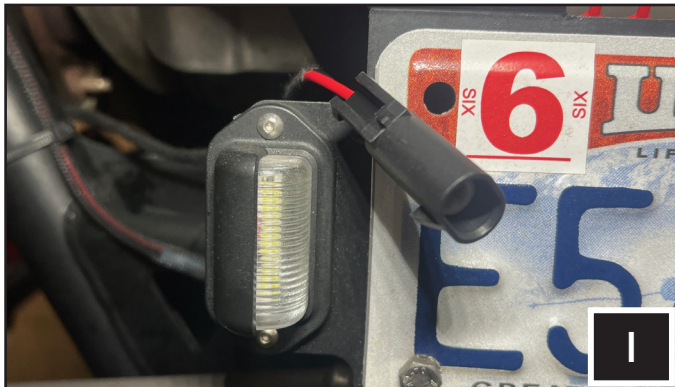
I. Run the "LIC. PLATE" connector towards the license plate location. Use zip ties to secure the cable away from any moving parts or the exhaust pipe.
