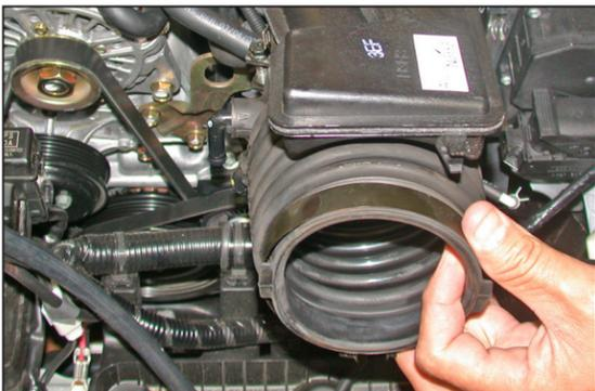
15. Remove the intake hose as shown.
