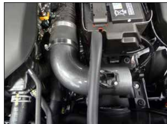
14. Route the K&N intake tube into the heatshield and then into the coupler, align for best fit and secure with the provided hose clamp.
