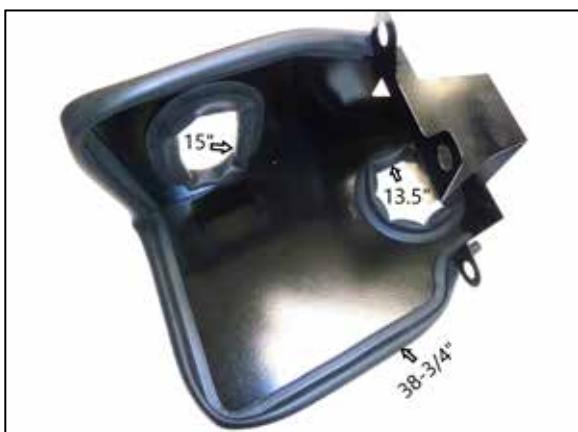
7. Cut the provided edge trim into sections of 38-3/4", 15" & 13.5" long then install the edge trim onto the heat shield as shown.
