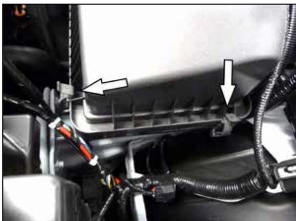
4. Release the two spring clips that secure the air filter housing lid, remove the lid and factory air filter.
