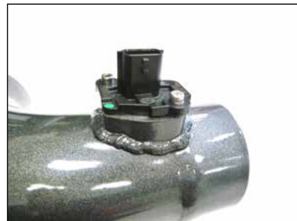
12. Remove the mass air sensor from the factory housing and install it into the K&N intake tube using the provided hardware.
