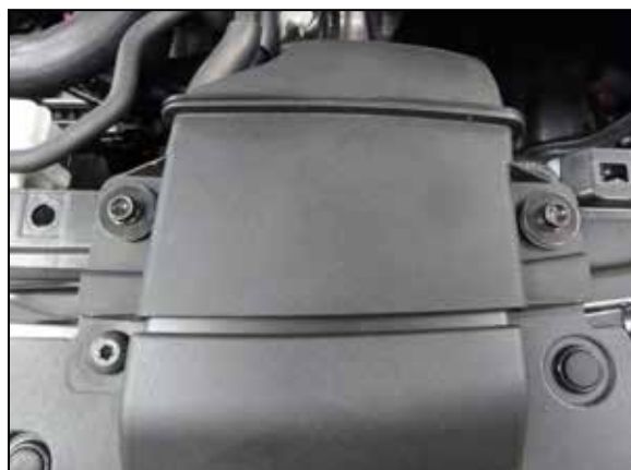
11. Re-install the factory bolts to secure the fresh air duct.
