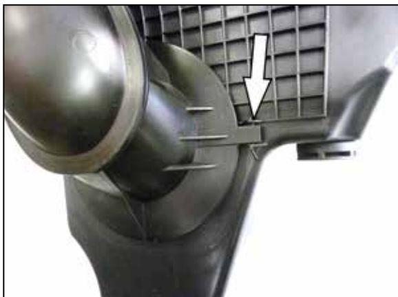
6. Release the locking tab then rotate the fresh air duct counterclockwise to release it from the lower air filter housing.
