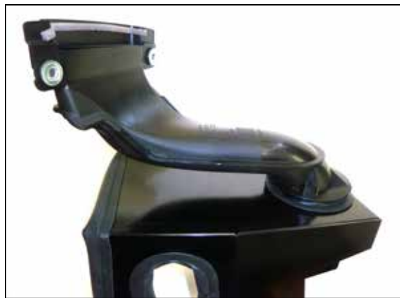
9. Install the fresh air duct into the K&N heat shield as shown.
