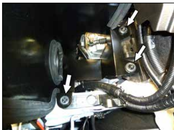
10. Install the heat shield assembly into the vehicle guiding the grommets over the mounting studs.
